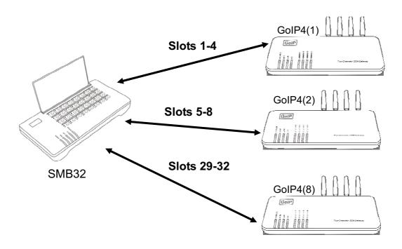
The card numbers of the remote-end devices corresponding to the cards on the "schedule mode = fixed mode" slots
