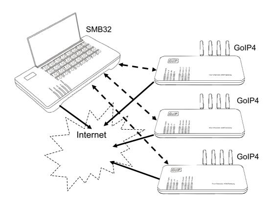
As shown in the above figure, several GoIP devices (up to 32 ways) can be connected to the SMB32 through Internet. The SIM cards installed with the devices are all integrated to the SMB32 to be controlled and scheduled by the latter. (SIM Bank mode: server mode)
