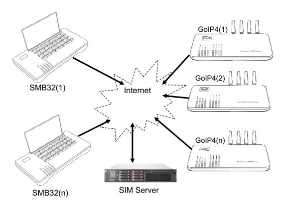
More than 10,000 SIM cards can be collectively scheduled and managed via the SIM Server. The planned tasks are allocated by the SIM Server (SIM Bank mode: client mode)
