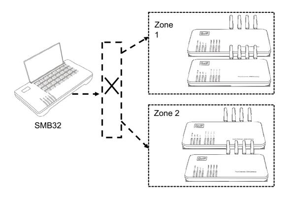
When schedule mode is used (schedule mode = schedule), devices of different zones will automatically exchange their SIM cards when it is time for schedule, so as to realize the automatic roaming of SIM cards. When this configuration is used, chaos mode is adopted for the relationship between the SIM cards and the remote-end devices.
